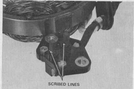
Remove and replace the brush with the mounting screws,
