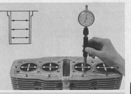
Inspect the top of the cylinders for warpage. Check in an X pattern as shown. SERVICE LIMIT: 0.25 mm (0.010 in)
