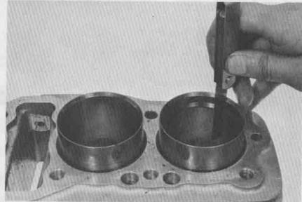
Insert each piston ring into the cylinder, and inspect the end gap.
