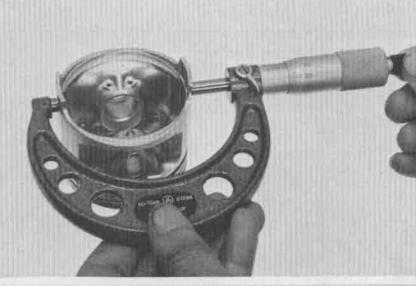
Measure the piston pin hole I. D. SERVICE LIMIT: 15.08 mm (0.594 in)
