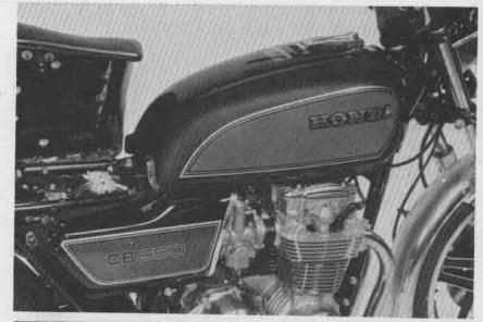
Disconnect the starter cable at the starter relay switch.
