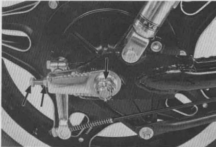
Remove the gearshift pedal. Remove the left rear crankcase cover.
