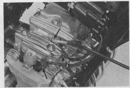
Disconnect the clutch cable at the clutch arm.
