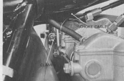
Remove the choke cable from the choke cable bracket on the handlebar holder.
